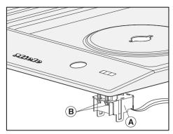
Carefully remove the upper section of the appliance. When doing this make sure you do not also pull out the light unit for the display (a) located underneath the upper section. To release the unit, squeeze together the two clamps (B).
